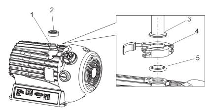
Fig. 6: Example of vacuum connection
