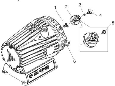
Fig. 21: Removing gas ballast valve
