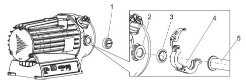
Fig. 7: Example of exhaust connection
