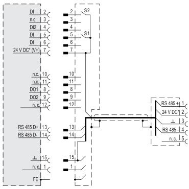
Fig. 11: Connection diagram of 15-pin "remote" connection
