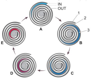
Fig. 2: Schematic compression cycle of scroll pumps
