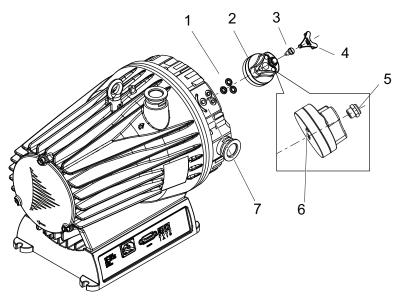
Fig. 24: Installing gas ballast valve
