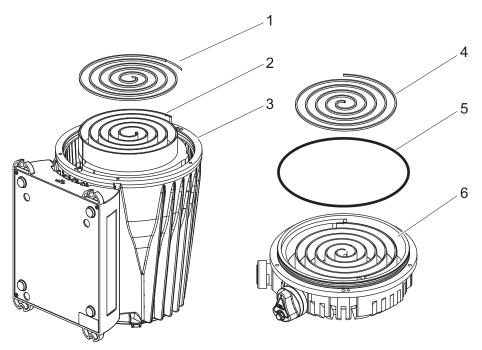
Fig. 28: Replacing the tip seal on the scroll pump
