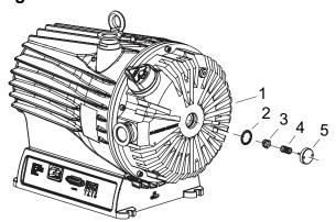
Fig. 19: Removing valve
