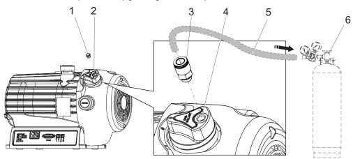
Fig. 8: Connecting gas ballast external supply
