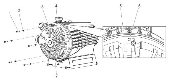
Fig. 27: Removing the scroll pump spiral housing
