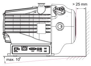
Fig. 5: Minimum distances and permissible inclination
