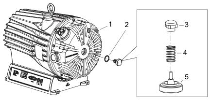
Fig. 20: Installing valve
