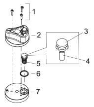
Fig. 23: Assemble gas ballast valve
