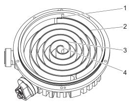
Fig. 29: Tip seal nut in the spiral housing
