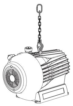
Fig. 4: Slinging points for transport of the scroll pump
