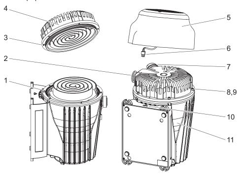
Fig. 30: Assembling the housing parts
