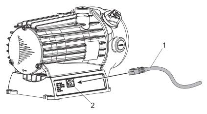
Fig. 9: Connecting to mains power supply
