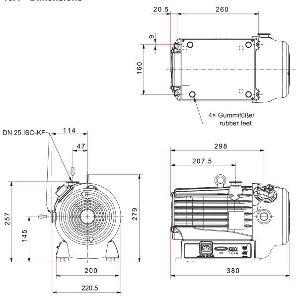
Fig. 33: HiScroll 6 | Version with pressure sensor
