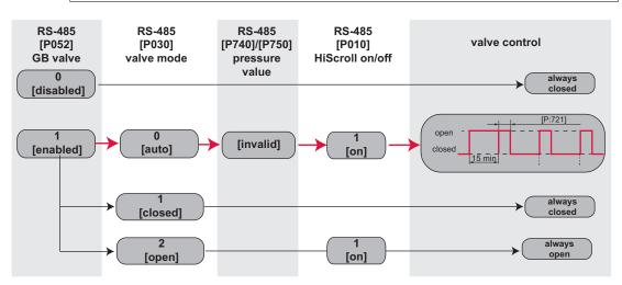
Fig. 18: Gas ballast valve control in automatic mode
